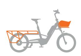
**FXAMPLE** VELO DE VILLE LOADY with Cargo Kit Pro 35 kg + Weight cyclist 75 kg 50 kg + Two children á 25 kg / approx. 8 years + Load on front carrier 5 kg **15** / **35** kg + Trailer<sup>1</sup> incl. load Total weight WITHOUT Enviolo HD 180 kg Total weight WITH Enviolo HD 200 kg 75 kg Position the load as centrally as possible on the rear carrier. 50 kg When transporting passengers, they should be seated further forward. 15/35 kg
