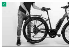
6. Make sure the saddle is not out of alignment using the top tube [a] or the bottom bracket shell as a reference. If necessary, open the clamping, realign the saddle and retighten the clamping [b].
