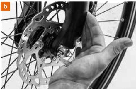
Move the lever back, as if to close it. Now you should be able to read "Close" on the outside of the lever. When you start closing the lever you should feel virtually no resistance with your hand until the lever is at right angle to the frame/fork.
