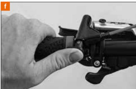
When you have set the sag correctly, as above described, and when the rear shock works properly during a normal test ride, but if then the rear shock bottoms out nevertheless, you can increase the compression damping a little.
