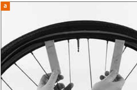
Before fitting the tyre completely on the rim check again whether the inner tube lies properly inside the tyre and press the last stretch of tyre over the edge of the rim using the balls of your thumbs.
