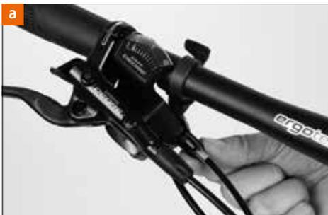
After tensioning the shift cable check that the chain immediately climbs onto the next larger sprocket. To find out you either have to turn the cranks by hand or ride your Velo de Ville bike and shift through the gears.
