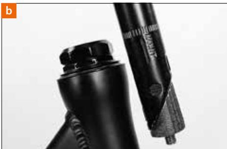
Now you can move the handlebar/stem-unit up and down as a whole. Be sure not to pull out the stem too far. The mark on the stem (end, min, max, stop, limit or the like) should always remain within the tube [b]. Setting the stem to a lower position can only add to your safety!
