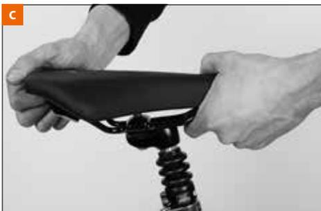
The preload is increased by turning the adjusting screw clockwise; this makes the suspension harder. The preload is reduced by turning the adjusting screw anticlockwise; this makes the suspension softer. The adjusting screw is at or in the end of the seat post tube and can only be reached when the seat post is removed from the frame. To adjust the saddle height, please proceed exactly as described above.
