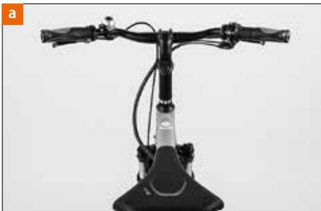
4. Make sure the saddle is not out of alignment using the top tube [a] or the bottom bracket shell as a reference. If necessary, open the clamping, realign the saddle and retighten the clamping. For more information see the chapters “Adjusting the Velo de Ville bike to the rider”, “How to use quick-release systems and thru axles” and the enclosed operating instructions of the component manufacturers.
