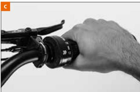
Depending on the gear system, gear shifting is initiated by actuating a shifter or by a short turn of the wrist with twist grips [c]. Continue pedalling during gear shifting, however, at reduced pedalling force.
