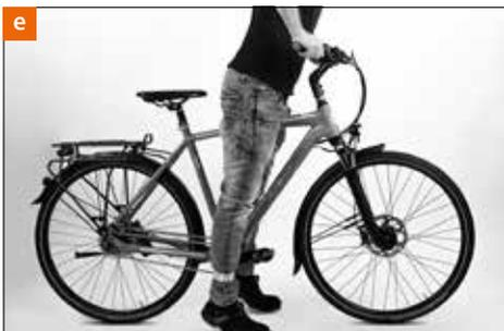
5. Let your Velo de Ville bike bounce on the ground from a small height. If there is any rattling, check where it comes from. Check the bearings and bolted connections, if necessary.
