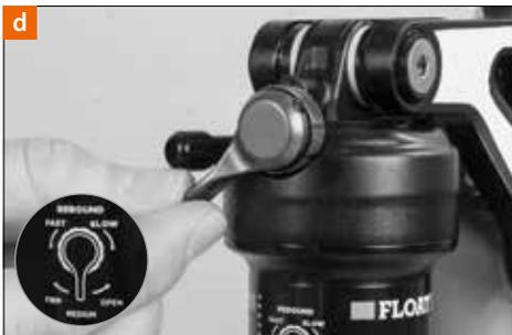
Ride over an obstacle (e.g. down a kerb) subsequently and turn the rebound damping in small steps towards the “+” or “slow” setting. You have found the proper rebound setting when the rear frame does not cycle more than once. Always check a changed setting during a test ride in the terrain.
