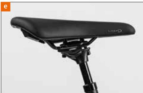
Tighten both bolts evenly [f] so that the saddle remains at the same angle. If you wish to lower the nose of the saddle a little, tighten the front bolt clockwise. You might have to loosen the rear bolt a little as well. To lower the rear part of the saddle, the rear bolt has to be tightened clockwise and the front bolt to be released, if necessary.
