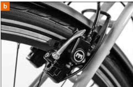
With rim brakes the sides of the rims also serve as braking surfaces [b]. An untrue wheel can impair the braking effect. Therefore, check the wheels from time to time for trueness. For this purpose lift the wheel off the ground and spin it with your hand. Watch the gap between the rim and the brake pads [c]. If the gap varies by more than a millimetre, you should ask a Velo de Ville dealer to true up the wheel.
