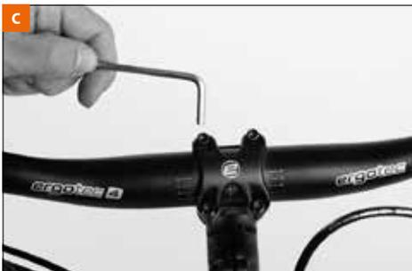
You can determine the handlebar height by the arrangement of stem and spacers **[b]**. Slip the remaining spacers onto the fork steerer tube above the stem. Adjust the headset, as described in the chapter “**Headset**”. When the seating position is as you want it, have the projecting spacer tower including steerer tube removed by your Velo de Ville dealer.
