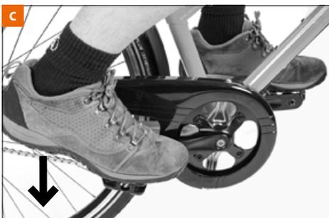
With multi-speed hubs normally the power transmission and the gear ratio adjustment is guaranteed via one or several planetary gears, depending on the number of gears. To change gears the pedal force should be reduced significantly for a short time.
