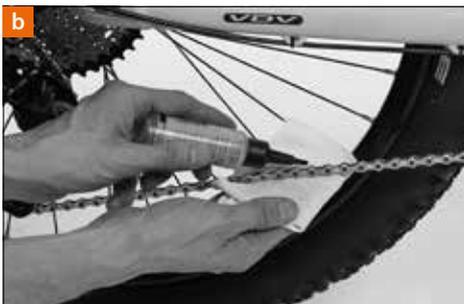
then let the Velo de Ville bike rest for a few minutes so that the lubricant can disperse. Finally wipe off excess lubricant with a rag so that it does not spatter around during riding or can collect road dirt.
