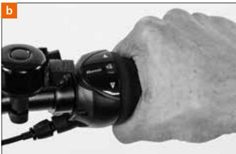
The advantages of multi-speed hubs [a] are their enclosed design. Unlike derailleur gears the gear drive is within the hub body, only the primary ratio from the chainring to the sprocket being outside. What is more, all gears can be shifted through with one gear shifter [b].
