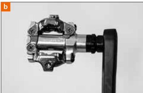
With these shoes small cleats are integrated into the sole which provide a firm hold on the pedal and yet at least satisfactory walking characteristics.
