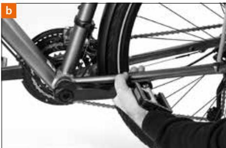
Also check at regular intervals whether the cranks are firmly attached to the bearing shaft or whether there is play. Grab the crank and try to jiggle it forcefully. It must be absolutely free of play [b]. If you notice any play, contact your Velo de Ville dealer immediately.
