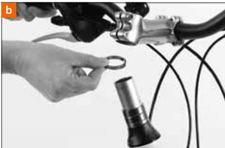
Unscrew the bolt at the top of the fork steerer tube which serves to adjust the bearing preload, remove the Ahead cap and release the bolts on either side of the stem by up to three turns **[a]**. Remove the stem and the spacers from the fork steerer tube. In doing so keep hold of both frame and fork to prevent the fork from slipping off the head tube.
