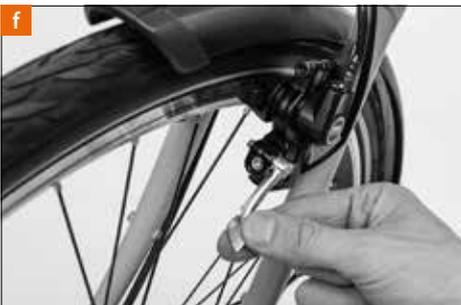
If your bicycle has **hydraulic rim brakes** from Magura, open their quick-release lever on one side of the brake [f] and remove the brake from the cantilever socket.
