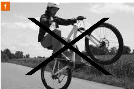
**Velo de Ville Trekking and Travel bikes [c]** are intended for use on normal, hard-surface ground, e.g. for tarred roads and cycle lanes as well as on unpaved roads and gravel paths of moderate classification. Under these conditions, contact with uneven terrain and the loss of tyre contact with the ground is possible. Steps or kerbs (jumps/drops) may only be performed up to a height of maximum 15 cm. The speed is 15 to 25 km/h (9.3 to 15.5 mph) in the average.
