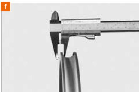
See your Velo de Ville dealer and ask them to examine the remaining thickness of the rims when you have worn through your second set of brake pads at the latest. Your Velo de Ville dealer has special measuring devices for determining the remaining thickness of the rims [f].
