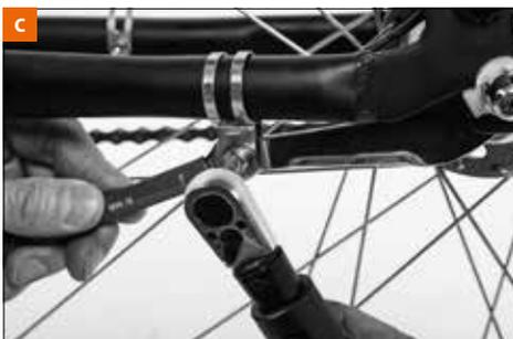
Tighten the clamp bolt of the brake arm to a torque value of 3–5 Nm [c]. Make sure the thread projects from the clamp nut by about 2–3 mm. If it does not, you need a longer bolt.
