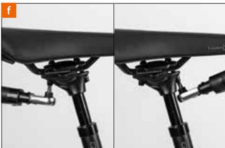
After fastening the saddle check whether it resists tilting by bringing your weight to bear on it once with your hands on the tip and once at the rear end.
