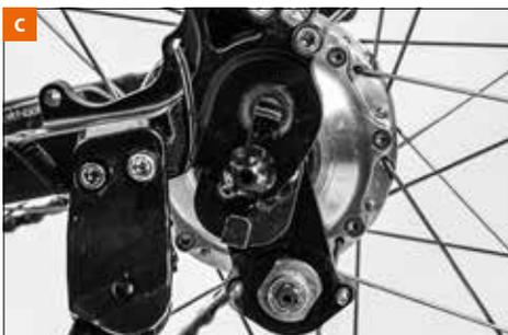
Loosen the quick-release lever or the lock nuts subsequently. Now you can take down the chain and remove the rear wheel from the frame [c].
