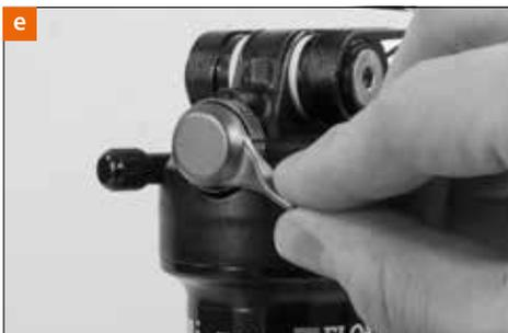
A weak damping ensures good response behaviour, may however lead under certain conditions (when riding too fast over obstacles, e.g. steps) to a too strong compression of the rear frame or to a bouncing when riding out of the saddle. A strong damping hardens the suspension, i.e. reduces the riding comfort.
