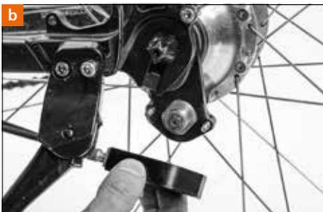
If you have a Rohloff hub with external activation, set gear 14 with the twist shifter first. After unscrewing the grooved bolt the gear box can be removed from its mount at the hub [b].
