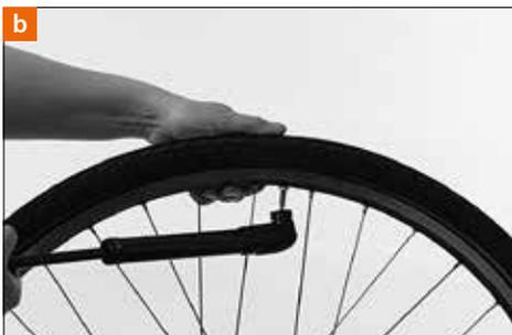
Push the valve a little into the tyre so that the inner tube does not get caught between the rim and the tyre beads. Check that the valve stands upright. If not, dismount one tyre side again and reposition the inner tube.
