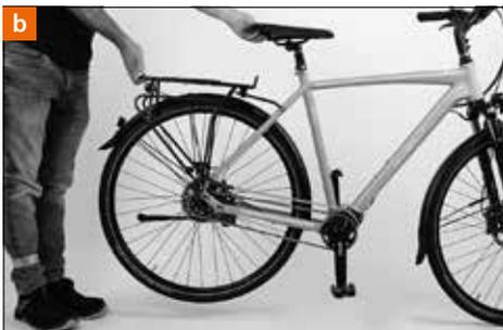
5. Lift your Velo de Ville bike up a few centimetres and let it bounce onto the ground [b]. If this causes any sort of noise, search for loosened bolts. Tighten them slightly, if necessary.
