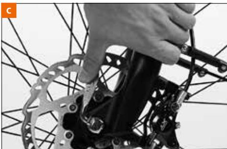
In its end position, the lever should be at a right angle to the quick-release axle, i.e. it should not stand out. The lever should lie close to the frame or the fork so that it does not open accidentally. Make sure, however, the lever is easy to grasp for an actually quick use.
