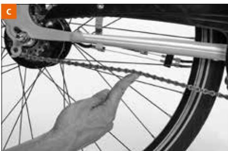
The cable tension is properly set when the ends of the shift cable housings are in the barrel adjusters without play, but unpressurised. The play of the twist shifter should be approx. 2 mm.
