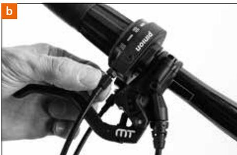
The play of the twist shifter is adjusted via the cable tension with the barrel adjusters. Unscrewing both adjustment barrels increases and screwing in both adjustment barrels reduces the cable tension and thus the play.
