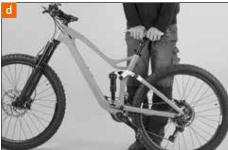
Then compress the rear frame several times [d] and wipe off excess lubricant with a clean cloth before you set off for your next ride.
