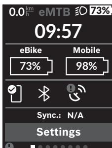
As well as the status bar, the status page also shows you the current time and the state of charge of all your eBike's batteries, as well as the state of charge of your smartphone battery if the smartphone is connected via *Bluetooth*®.
