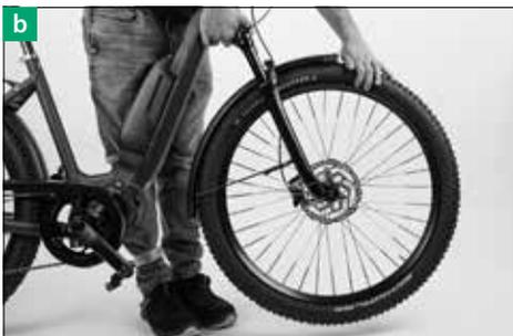
6. Are the tyres in good condition and do they have sufficient pressure [a]? Note that a Velo de Ville EPAC weighs heavier and that your usual tyre pressure may be insufficient. A higher pressure gives a better riding stability and reduces the risk of a puncture. The minimum and maximum pressure (in bar or PSI) is indicated on the tyre side.
