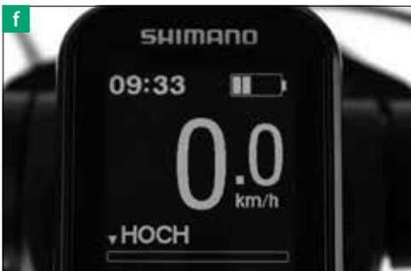
To extend the range it is recommended that you ride with low or no assistance at all on level or downhill trails and only select maximum drive assistance [f] with headwinds, heavy additional loads and/or when climbing hills.
