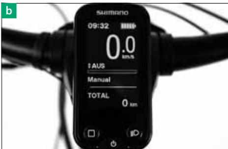
2. Check the display [b]. Are all values displayed as usual? Do not use your Velo de Ville EPAC, if the display shows an error message or a warning. If necessary, switch off the system and wait ten seconds at least before you check it again.
