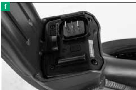
After you have removed the battery of your Velo de Ville EPAC from the down tube or the pannier rack: Keep the connections of the rechargeable battery [f] free of dirt and moisture. Protect the connections of your rechargeable battery with the protective covers, if supplied. With the battery removed the display and in particular the lighting system will, however, no longer work. Do not use your Velo de Ville EPAC on public roads any longer.
