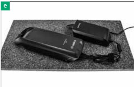
4. The rechargeable battery of your Velo de Ville EPAC must be charged before you set off for the first time [e]. Are you familiar with the handling and mounting of the rechargeable battery? Before you set off for the first time, check that the battery is properly mounted, that it has engaged audibly and that it is locked.
