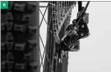
5. Check that the chain still runs on the chainrings and the sprockets. If your Velo de Ville EPAC fell over to the chain side, verify the proper functioning of the gears. Ask somebody to lift your Velo de Ville EPAC by the saddle and carefully shift through all the gears. Pay particular attention when shifting to the small gears and make sure the rear derailleur does not get too close to the spokes [e+f] as the chain climbs onto the larger sprockets.
