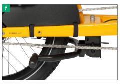
10. Check all add-on and accessory parts, such as the rear and the front pannier rack, front basket, child seat, trailer device etc., by trying to gently move the parts back and forth to check their tight seat. If the parts are not tight, realign the components and gently tighten the bolts until they are fastened securely. If you are in doubt or if you have any questions, contact your VELO DE VILLE dealer.
